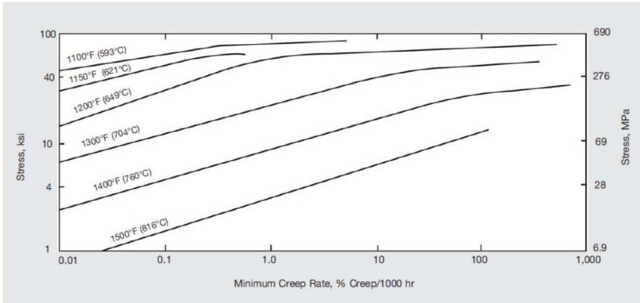
Figure 13 – Creep strength of annealed material.
