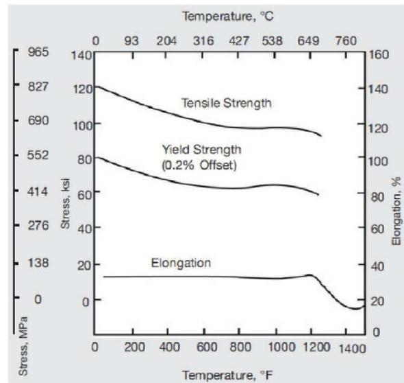
Figure 20 – High-temperature tensile properties of alloy 625
