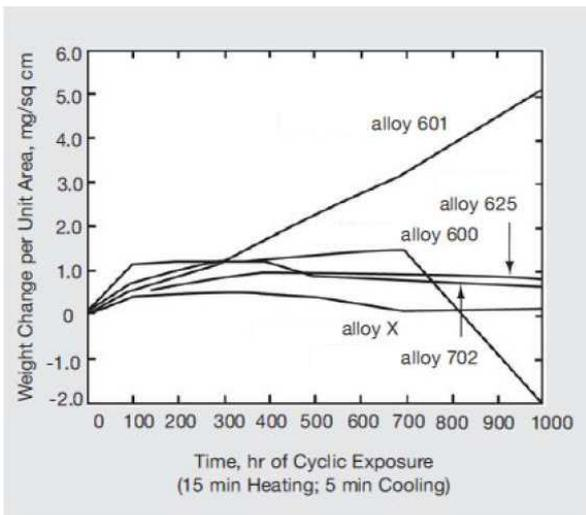
Figure 15 – Scaling resistance at 1800°F
