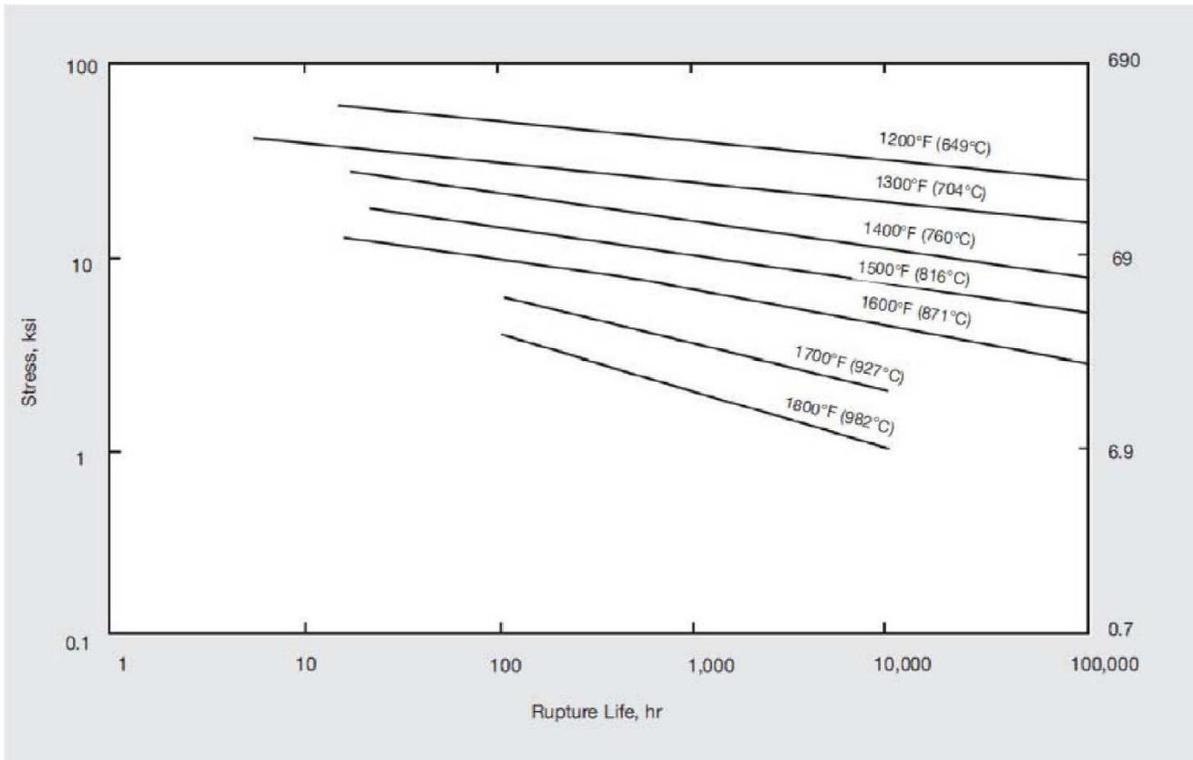
Figure 22 – Rupture strength of Welding Electrode 112 all-weld metal.
