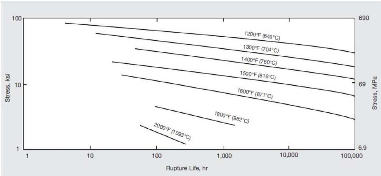
Figure 12 – Rupture life of solution-treated material.
