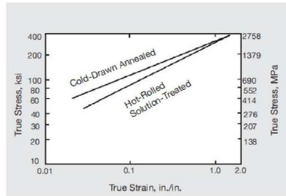
Figure 2 – True stress-true strain of round.
