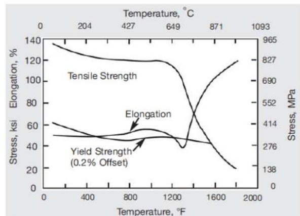
Figure 4 – High-temperature tensile properties of cold-rolled annealed sheet.
