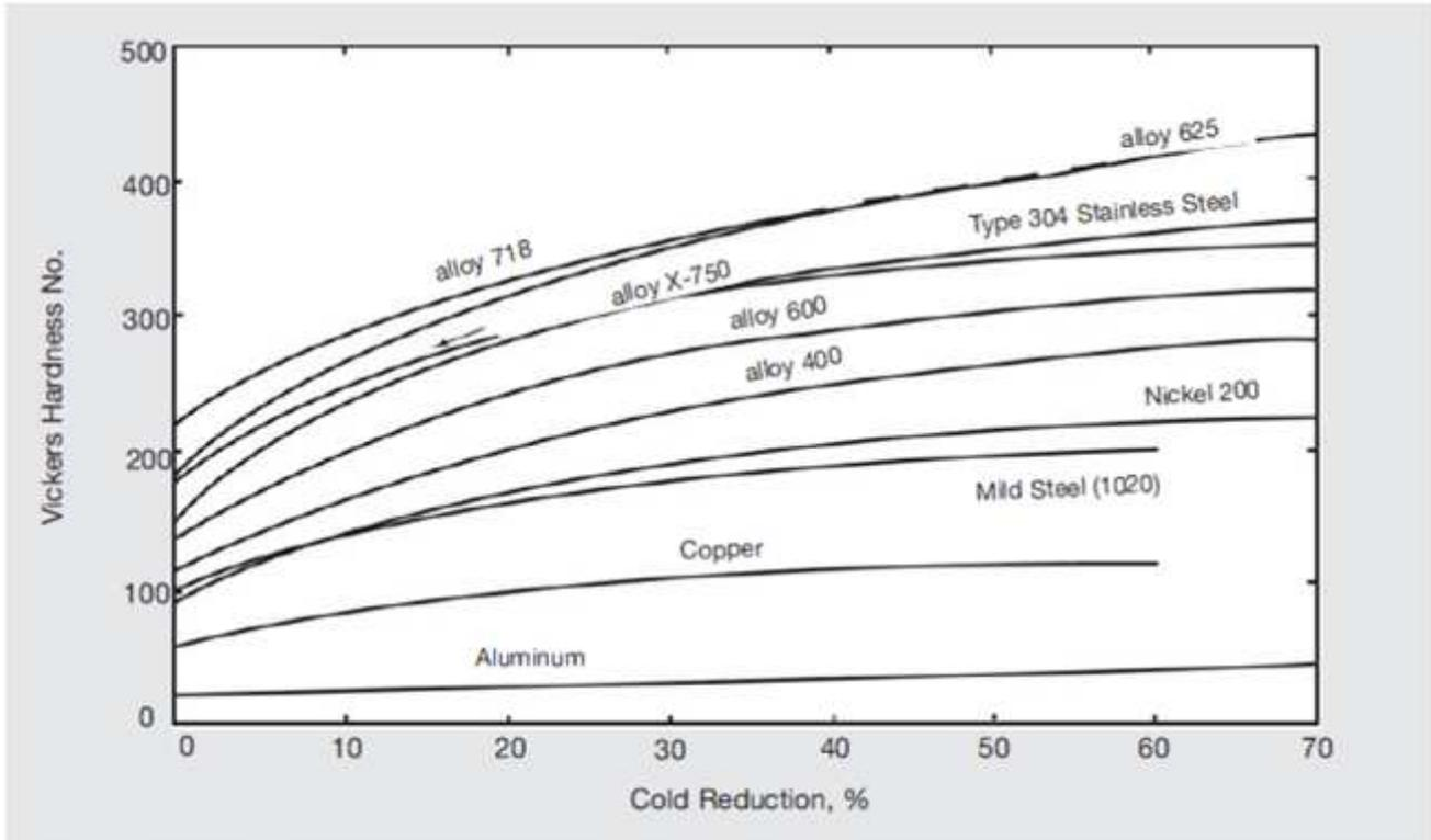
Figure 18 – Effect of cold work on hardness.
