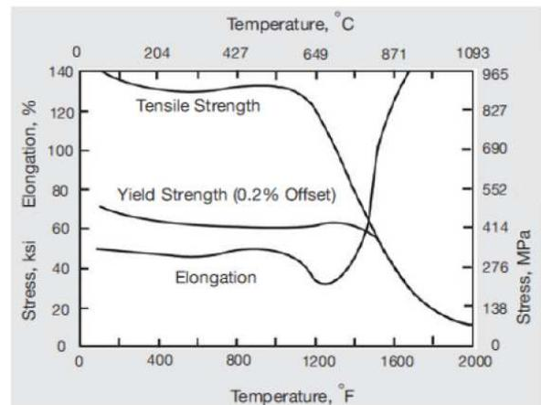
Figure 3 – High-temperature tensile properties of annealed bar.
