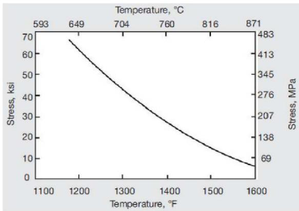
Figure 23 – 100-hr rupture strength of transverse specimens from joints alloy 625 made by gas-tungsten-arc process.
