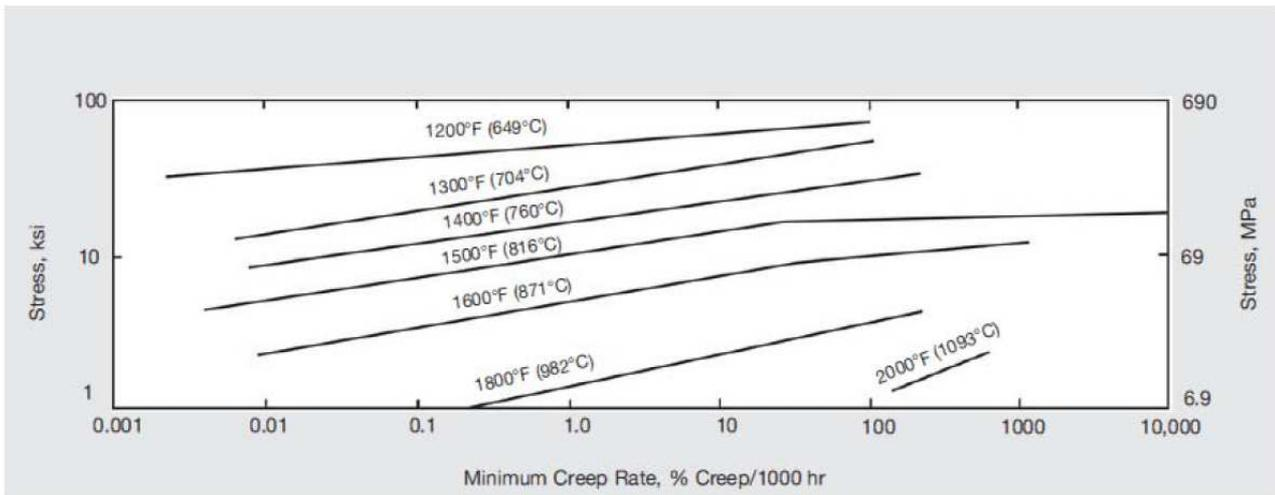
Figure 11 – Creep strength of solution-treated material.
